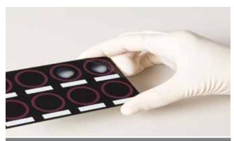
5. GENTLY ROCK THE TEST CARD BACK AND FORTH FOR 3 MINUTES THEN EXAMINE THE REAGENT AND SAMPLE IN THE CIRCLE
