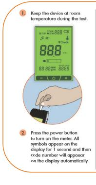
Insert the test strip with the G6PD side facing up until it does not enter further anymore. A beep will sound. When the blood symbol flashes on the standby mode, preparation for the test is done.
